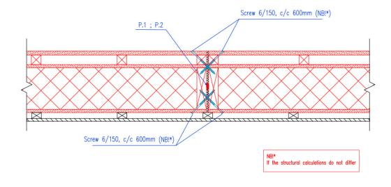
P.1 Montage gap 10 mm.P.2 Gap sealing Ø16 mm + Foam insulation
